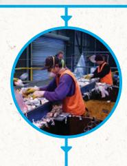
The recyclables are sorted into different material types by hand and machinery.
