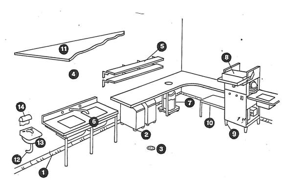
FIG. 2. Requirements — Typical Wash-up Area
