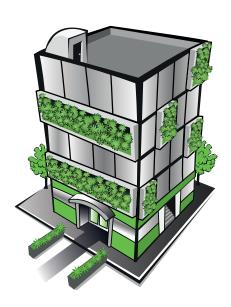
We know the city can be 4 to 7 degrees hotter than surrounding suburbs due to the urban heat island effect. Green walls, facades and rooftops not only look good but help cool our city and retain stormwater which can help reduce flash flooding.
