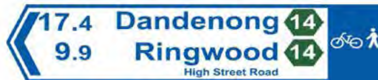
Figure 7.5 An example of a standardised trail directional sign type, including route numbering (adapted from Finding Melbourne: Standardising Melbourne/Victorian Bicycle Wayfinding Systems, Chris Hui, & Winchelle Chuson, 2012)
