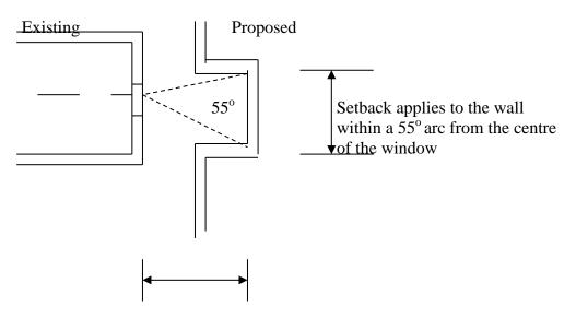
Wall setback from the window half the height of the wall if wall exceeds average height of 3.0m
