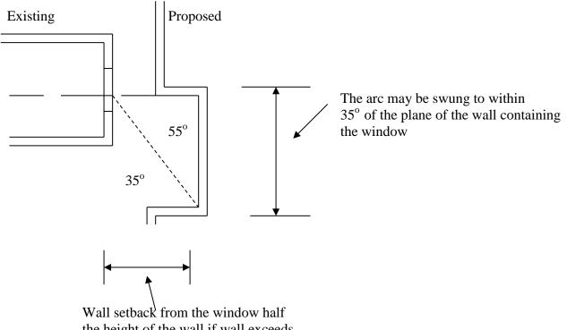
the height of the wall if wall exceeds average height of 3.0m
